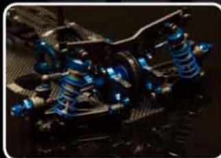
Adjustable differential height and belt tension Blue titanium turnbuckles Blue aluminum clamping wheel hexes
