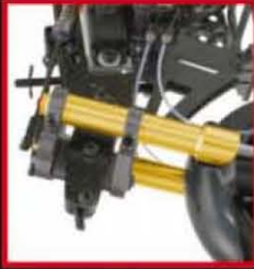
ALLOY FORKS WITH ADJUSTABLE PRELOAD
