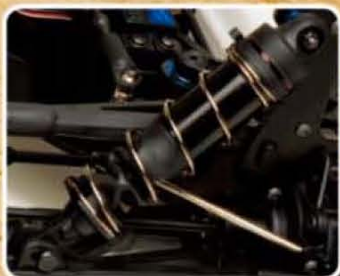
Composite 'Big Bore' 16mm shock bodies and caps. 4mm shock shafts with protective rubber boots.
