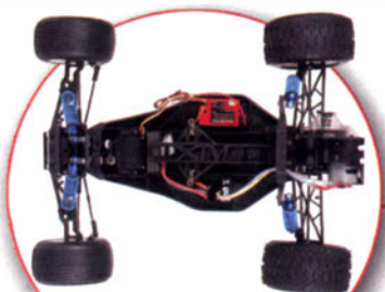
Reinforced Molded Composite Chassis
