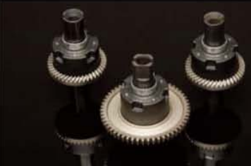
RC8T differentials come preassembled and ready to fill with diff fluid
