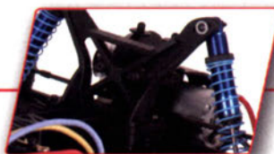
Fully Threaded Aluminum Shocks
