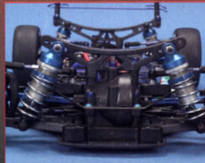
Shims under the suspension blocks are used on asphalt and removed when on carpet.
