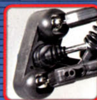
The Ultra MBX Comp comes with pivot ball suspension and a 330mm wide arm set.
