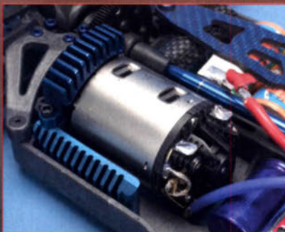
Once again the signs of some Factory Team parts. The extra cooling of the machined aluminum is useful.
