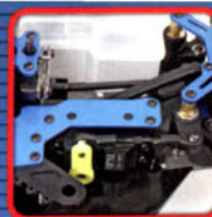
Both buggies include lay-down servos and blue anodized aluminum hop-ups installed.
