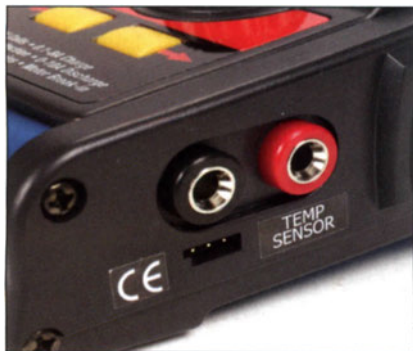
The charging leads have banana-plug inputs, and an optional temperature probe can be added.
