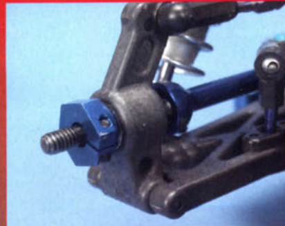
Barry uses the Factory Team aluminum hexes for a little extra durability.
