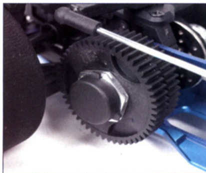
The slick shifting 2-speed has a wide array of optional gearing choices available through RD Logics.
