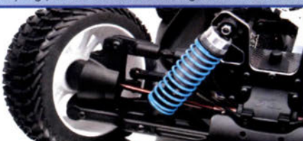
Composite steering block with molded-in steel bushing.
