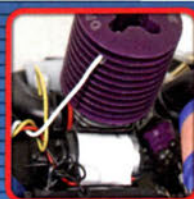
The Ultra MBX Comp includes a powerful .26 engine with OFNA's electric start system.
