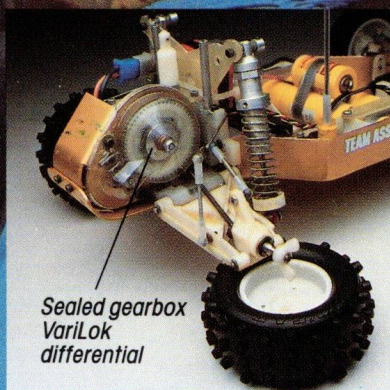
Full race rear suspension includes bulletproof half shaft and u-joints with tapered and keyed modular wheels. Quick release knock off design for fast pit work and tuning.
