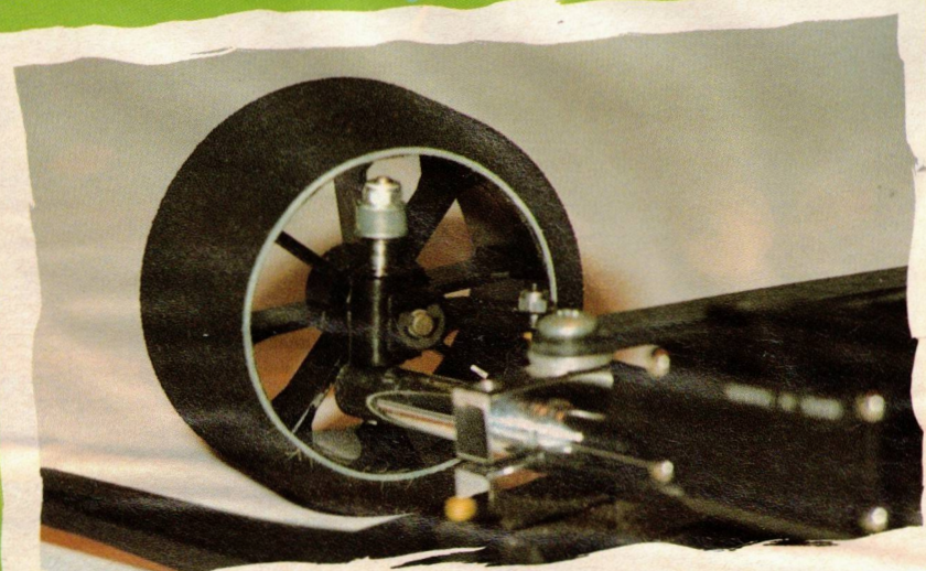
Hyperdrive's exclusive "no bumpsteer" servo mounting system has the servo mounted on a tray that is attached to the axle (above and below).
