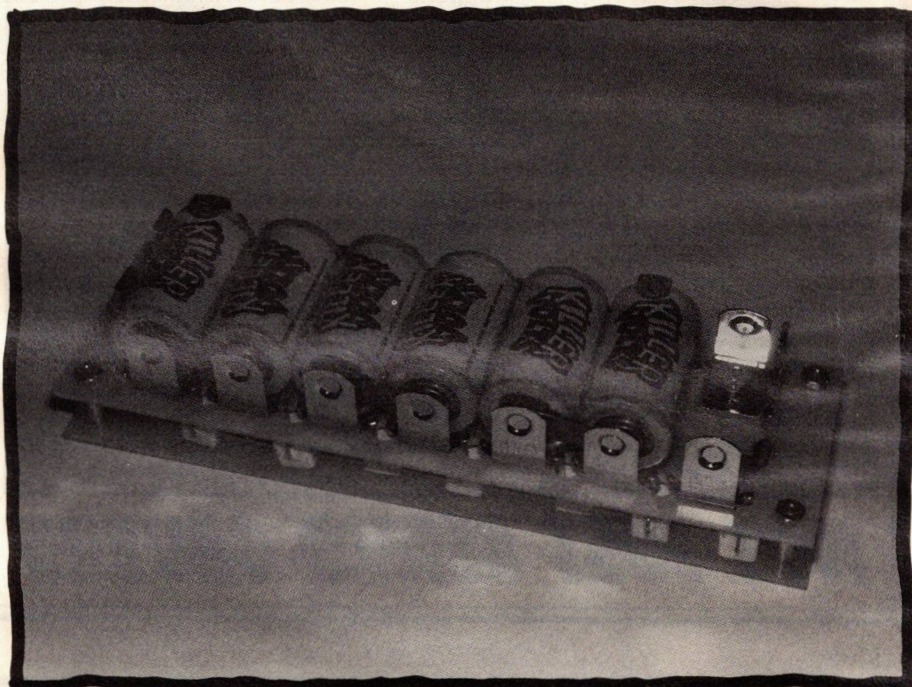
Above, a race pack is placed into the Drop Quick discharger, allowing each cell to discharge individually. Once the pack has cooled, it is removed for charging when needed.
