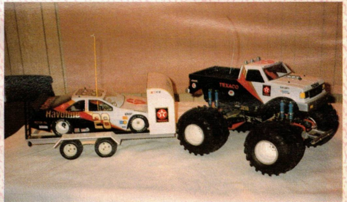
Doug Clark's Clodbuster is pulling a homemade trailer that Doug built from scraps in his shop. The undercarriage is hardwood from an old hockey stick, and the axles were made from a lawn ornament and tires and rims were off an old RC10.
