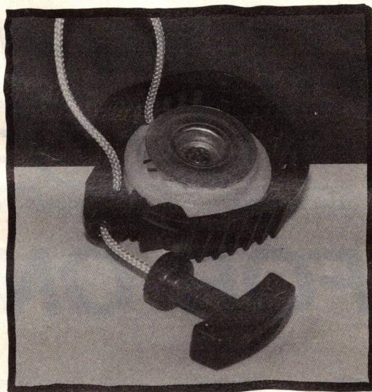
This is the Zenoah pull starter. Notice the loop in the photo. This is to hold on to for loading and unloading tension on the starter spring.
