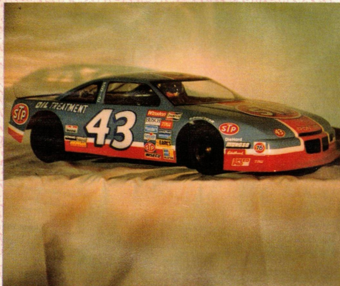
Richard Petty's Pontiac racer has been recreated in 1/10th scale by Leon Fahrenthold, of Anchorage, Alaska, using a Pro-Line Grand Am body over a TRC Lynx II Elite chassis. Additional equipment include a Tekin ESC, Futaba radio, and a 12-turn Single Reedy Blue Dot for speed.
