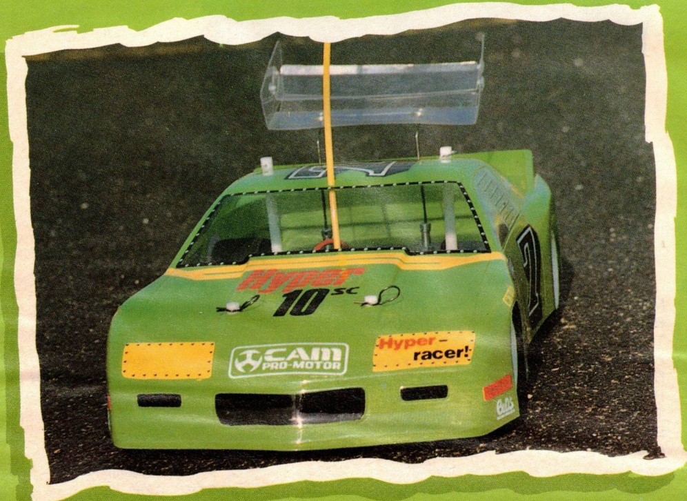
Above and left: The 10SC shown here has the BoLink '89 IROC Camaro body, CKW capped tires, and a Bud's Airflow wing as standard equipment for superspeedway contests.
