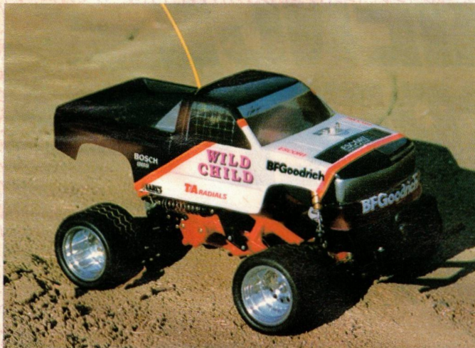
A Wild Child, from Michael Ford, of Visalia, California is a Blackfoot with Andy's body, oil-filled shocks, Sees aluminum wheels, Thorp rear end, gears, dogbones, and more. The motor is a Race Prep, with Futaba radio gear and ESC. Mike says it's good-looking, and fast too!
