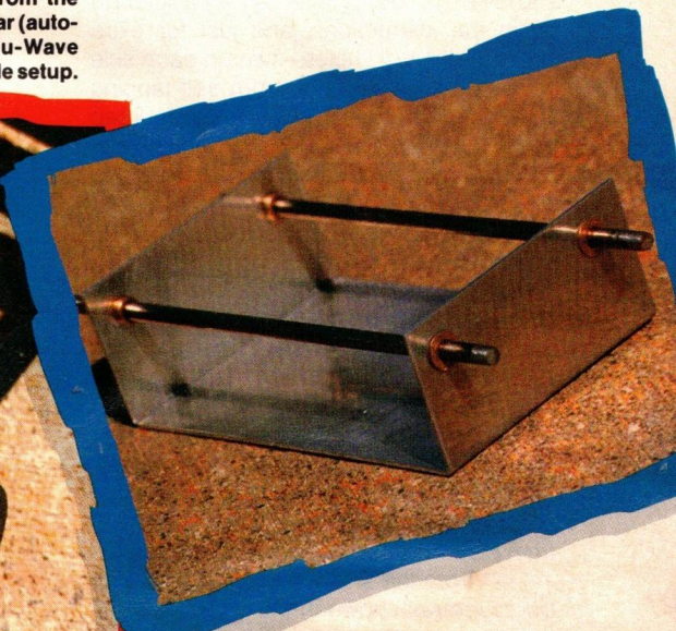
Above, this is how your rear axles should look once you've completed this task. Jack used aluminum sheet, .50-inch gauge, instead of the plastic or Kydex recommended in the instructions. Diagrams for making the necessary parts are on the following page.
