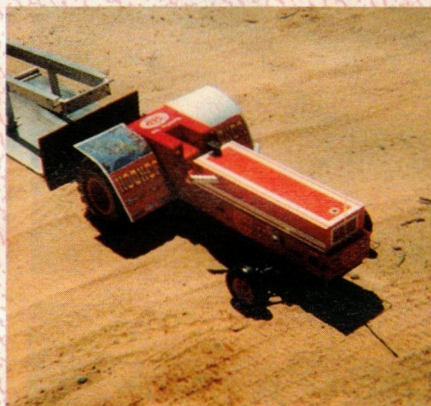
Next in bizarro class is this tractor made of aluminum bar stock with a modified Grasshopper tranny, Monster Mash motor, and an aluminum sled. It has pulled 75 pounds on grass, and the owner, Richard Hooker, of Stanton, Michigan, says the weight box will top out at 25 feet.
