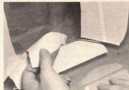
Thoroughly wipe out the inside of the body with denatured alcohol, then use wide masking tape and a hobby knife to mask the windows.
