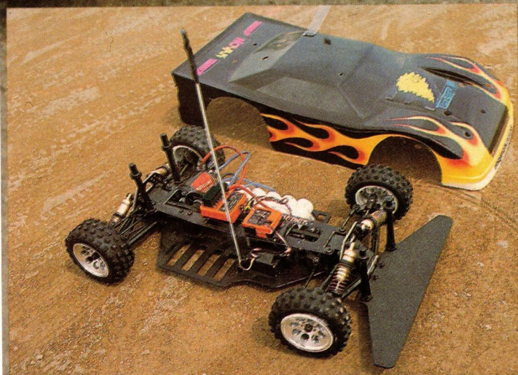
The 4WD Slingshot comes with high-quality bearings, Kyosho gold shocks, and a light fiberglass chassis.
