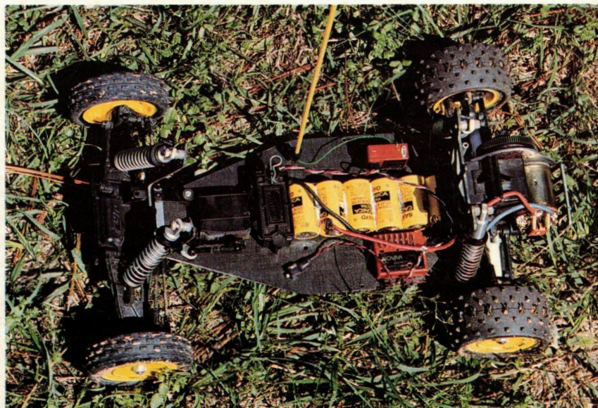
Steve Dunn's JR-X2, a duplicate of Mike Dunn's car, featuring Race Prep motor and batteries, and a Novak ESC. Mike won 2WD Modified class.
