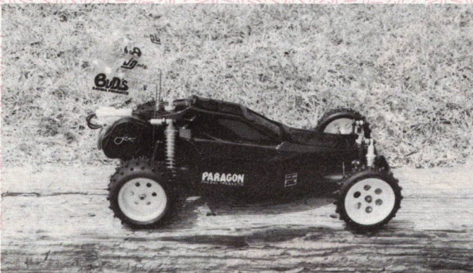
Here's a much-modified Ultima with a custom fiberglass chassis using Losi bell cranks and RC10 caster blocks, plus rear Option House shocks and CRP fronts. A Tekin ESC and receiver, and a Futaba mini-servo handle the control. It belongs to J.D. Wilson, Midwest City, Oklahoma.
