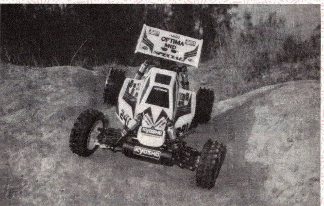
This Turbo Optima Mid SP has a LeMans 240 SB motor, a Futaba ESC, and an internal torque limiter to prevent motor damage if the wheels jam. It's from Hsi Lin, 16 years old, from Santa Barbara, California.
