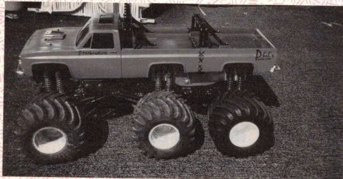
Greg Thomas, from Pinellas Park, Florida, says he named his Clodbuster "Frankenstein" because it has three Trinity Monster modified motors, Novak ESC, and Universal Energies power pack. The ESC is cooled by additional heatsinks and a hair dryer fan powered by its own 6-cell pack. Six wheel, six drive!! It's nuts!!
