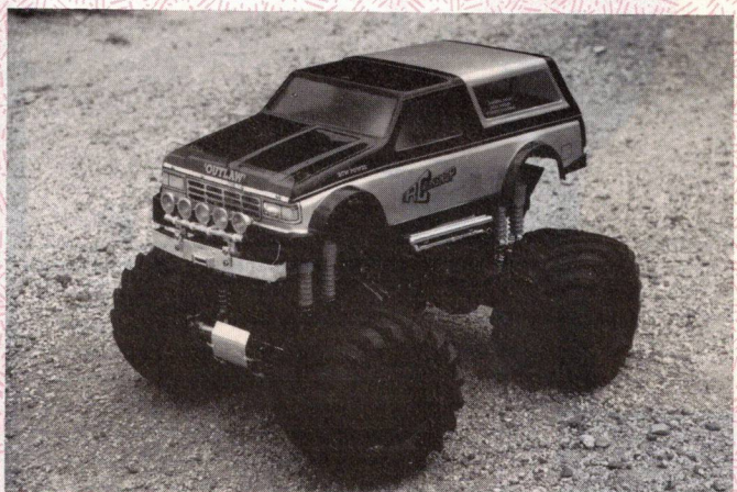
Cool-looking outlaw 'Buster from Brian Anderson, of Burlington, North Carolina. His truck has two Twister motors, Hornet speed controls, 2 8.4 battery packs, and 8 Tamiya shocks. Brian runs working headlights on his clean machine.
