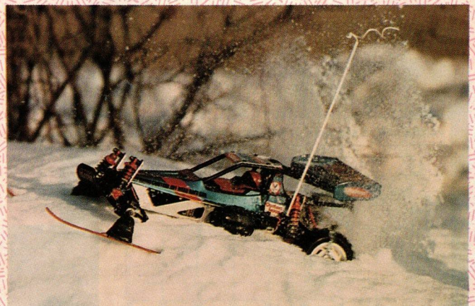
Josh Dodge, of Carbondale, Illinois, sends us this photo of his custom Ultima with skis and chains. Josh designed the skis and chains, with no help from a kit. The modifications keep his Ultima cruising through the winter. A free subscription is plowing its way to Josh.
