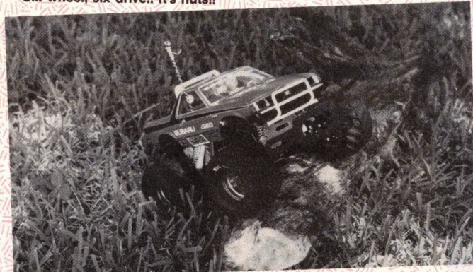
This Monster Beetle with a Brat body has a Diamond sprint motor powering it, and JG shock mounts. The paint job is by Bill Leary's mom, and the Beetle belongs to Bill. They're both from Boca Raton, and Bill says he probably could have painted it too.
