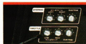
Servo reversing, throw adjustment and sub-trimming can be individually preset on the 2PD control panel.
