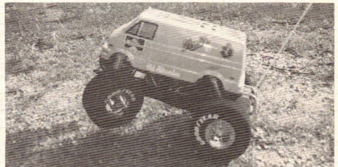
Joe Taylor, from Pomona, New Jersey, says he bought his father-in-law's Falcon and converted it to a Lunch Box called the Milwaukee Mudslinger. It has Twinn-K tires with Monster Beetle rims, a Trinity motor and a heavy-duty steering kit. A real wheelie beast!
