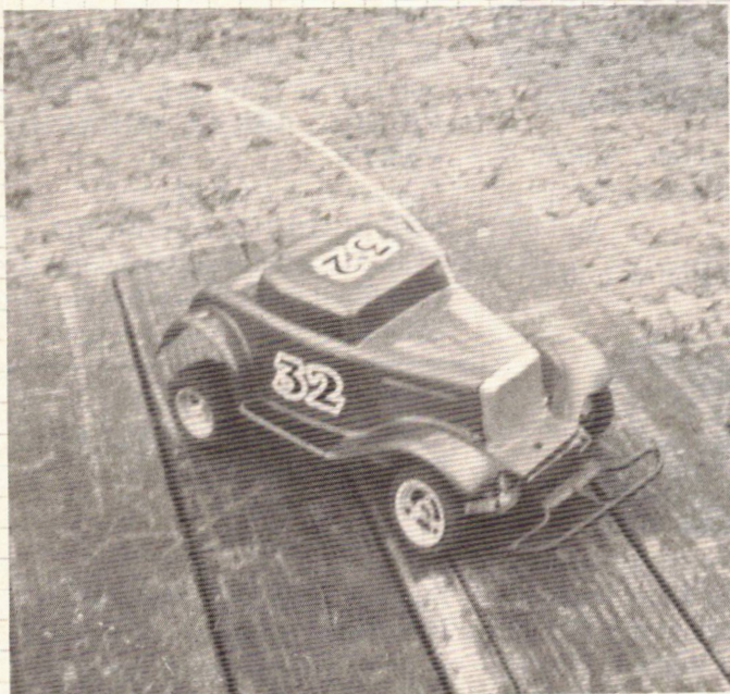
David Edwards, of Hudson, Florida says he runs his RC10 with a '32 Ford body in Late Model Modified class, with a Losi Insane motor, a Futaba speed control and radio, with high-speed servos.
