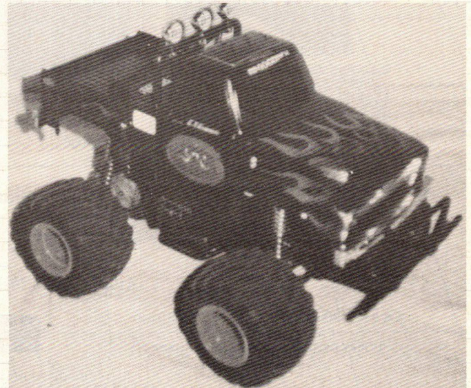
Greg Gale customized his Midnight Pumpkin with monster tires, a wheelie bar, tinted windows, working headlights, speed control, CVA long shocks, and a RS-540SD motor. The paint job took 3-1/2 days.
