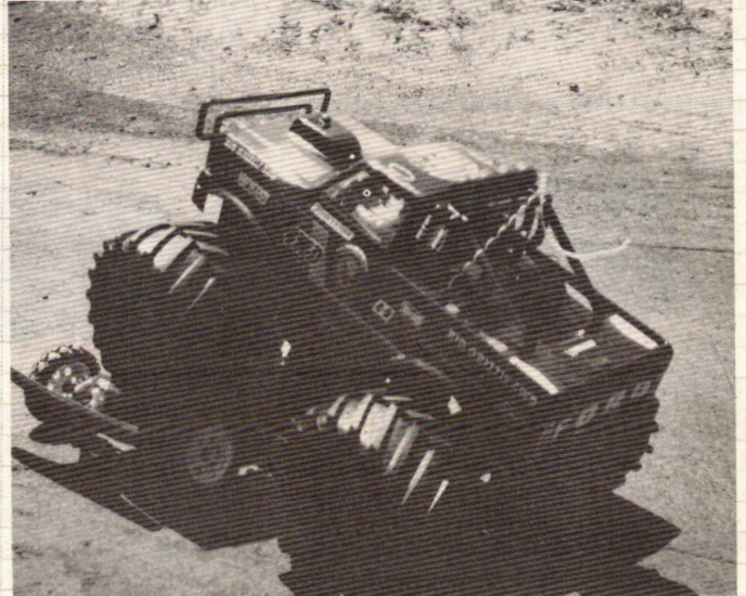
Stan Moxley writes to say that his Big Grizzly is completely stock, with an RS540 motor, and a Futaba radio.
