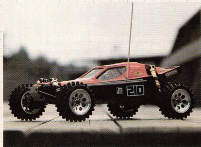
This Turbo Optima with a belt drive, low profile tires, aluminum rims, Novak speed control, Turbo racing battery, SPA 240WS motor, and gold chassis is from Chris MacQuarrie of Coquille, Oregon.
