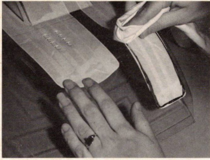
Wipe off your outside Sharpie guide lines now using denatured alcohol.
