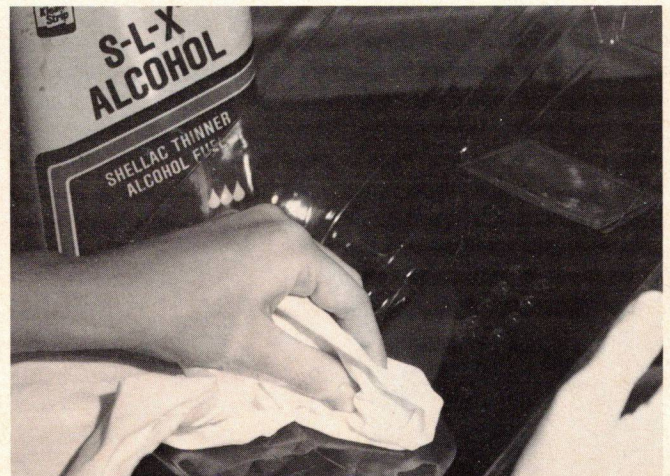
Use denatured alcohol to thoroughly wipe clean the inside of the car body before taping or painting. Use a clean, dry cloth to wipe.
