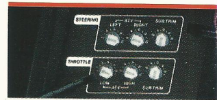
Servo reversing, throw adjustment and sub-trimming can be individually preset on the 2PD control panel.
