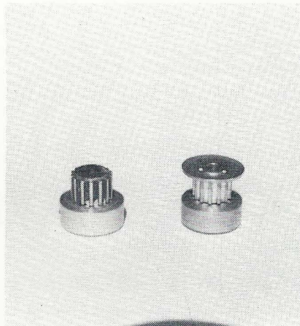
Left - Photo 6: The last modification. Remove the flange from the pinion. Right - Photo 7: On the left is the stock pinion gear. On the right is the modified pinion.
