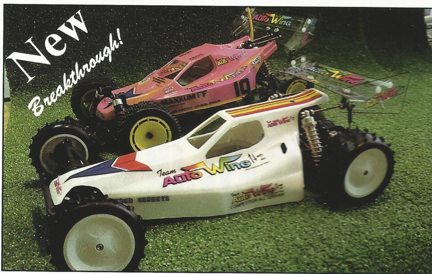
AUTO WING'S response to cornering . . . Here the wing angle changes to enable the car to hug the corner.
