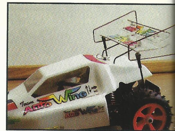
AUTO WING'S response on a Straight . . . Here the Auto Wing assumes an angle that provides the least amount of air drag.
