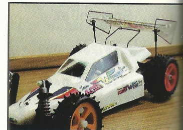
AUTO WING'S response to bottoming out . . . Here the Auto Wing temporarily assumes a lifting angle to keep the rear of the car from touching the track.
